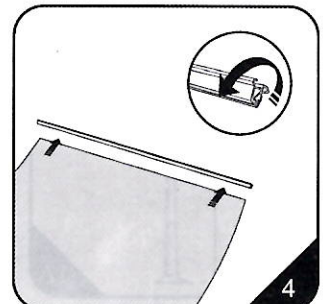
4. Open the top clip bar then insert the top edge of the graphic.
