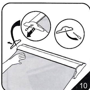
10. Peel off the left cover, remove the screw underneath the chrome end of the base and detach. Then, with the graphic held firmly, carefully pull out the retaining pin, then put it into the cover.
