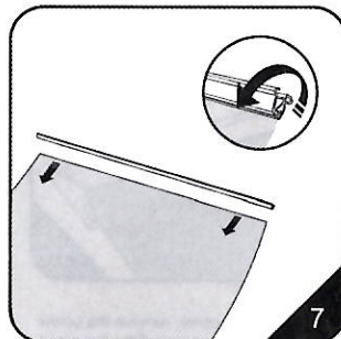
7. Swing open the beam's locking lip in order to relax the top edge of the graphic.
