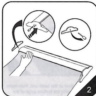
2. Pull the retaining pin out from the cover then carefully put it into the hole where the retaining pin was pulled out. (It may be useful to have an assistant)
